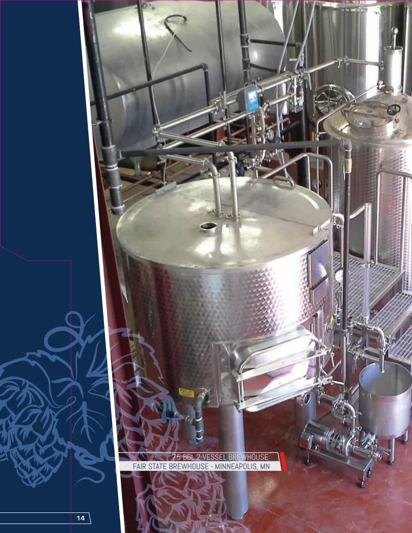
We grind smooth. We polish, and passivate every TIG weld. You can be confident that tanks look and perform as well inside as out. The largest possible stainless steel sheets are joined and butt-welded to create a stronger tank with fewer joints.
